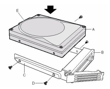
Figure 26: Installing the Hard Drive
